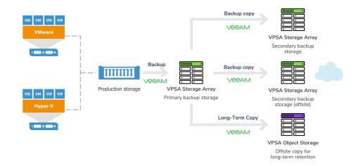
Zadara provides Veeam users the option to create a scalable, cost-effective backup repository comprised of multiple tiers of storage, to optimize for performance or capacity. The Zadara solution addresses Veaam's Performance Tier and Capacity Tier demands.
