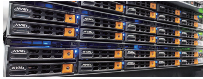
All NVMe Ceph Cluster (over 30node/1PB)
