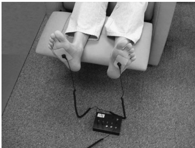
FIG. 1. Grounding system showing patches, wires, and box connecting to a ground rod planted outside through a switch (not shown) and a fuse (not shown). Similar patches and wires from the hands were also connected to the box to ground the hands.
